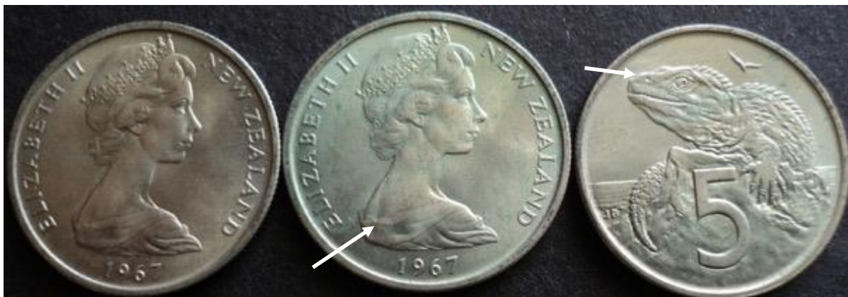
Obverse Hairline Die Crack and Reverse Die Crack through the Tuatara's head
