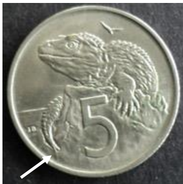
Die Crack and Cud on the Tip of Tuatara's tail
