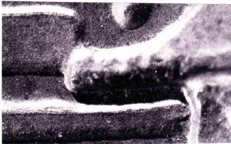
**Illustration 8** Minor recutting under Hobson's hat, reverse of coin D (die 2)
